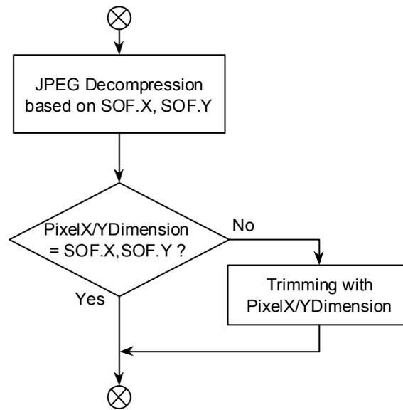
**Figure 37 Procedure for Image Data Reproduction**
