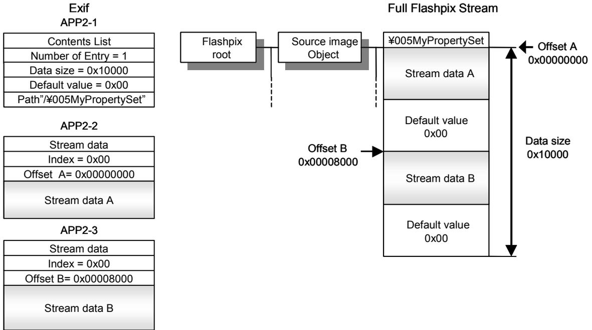
**Figure 62 Conversion to Flashpix Extensions (2)**
